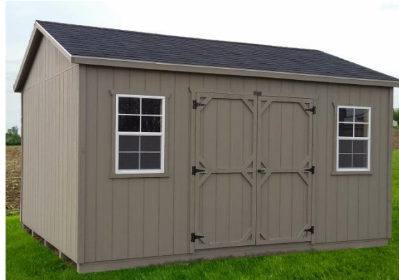
7' Sidewalls, 5' Double Doors, 5/8" Plywood Floor
